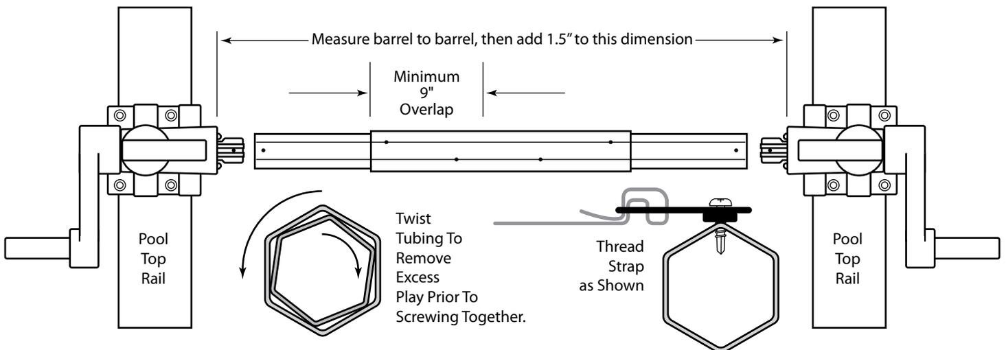
9. Attach Straps to Tubes: Come in 6 inches from each tube end and attach a strap plate to the aluminum tube assembly. Use the self drilling screws on the drill line to attach the plate. Look at the holes that were pre-drilled at the factory and use the same drill line. There are 6 lines on each tube. Take the remaining strap plates and connect them evenly along the length of the tube assembly. Attach Straps to strap plate. (See Illustration Above Right)
